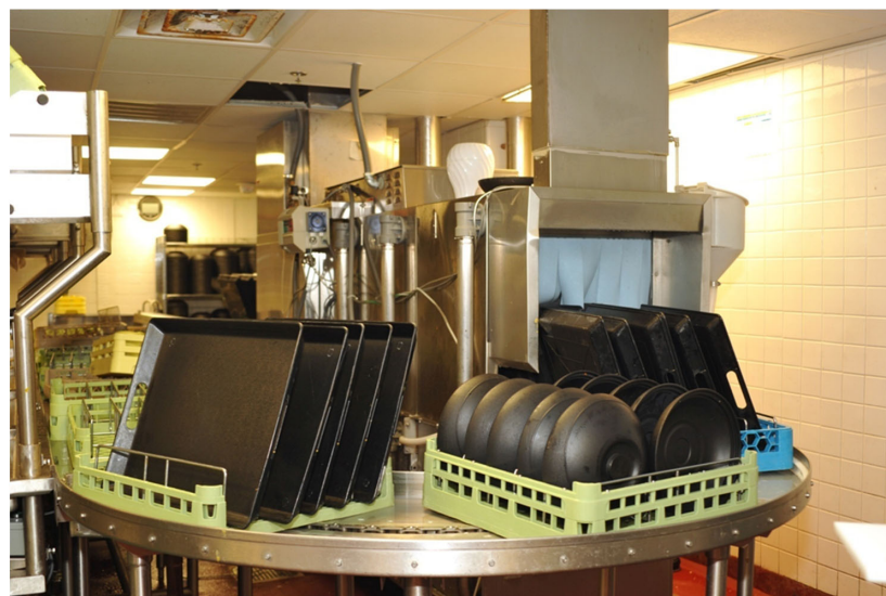
Automatic Washer-150°F wash for 20s, 180°F rinse for 10s
