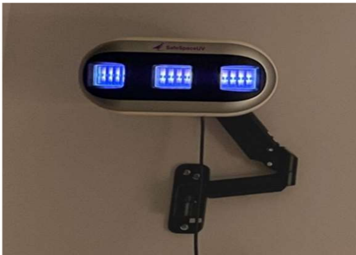
Figure 1. Picture of the wall-mounted device showing the 3 krypton-chloride excimer lamps and adjustable arm that can be used to adjust the position of the lamps.
