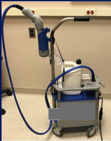
Picture of electrostatic sprayer (0.25% sodium hypochlorite)
